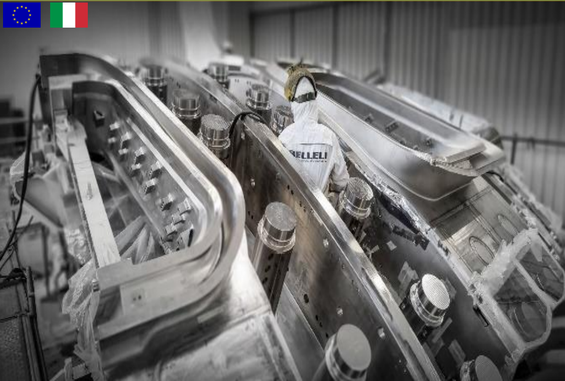
Five vacuum vessel sectors are under fabrication in Italy (Ansaldo Nucleare, Mangiarotti, Walter Tosto). Completion rates range from 76 to 97%
